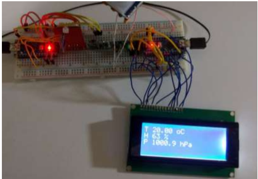
The breadboard with LCD display added
